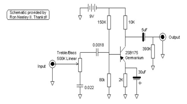
Another treble/bass booster, very much like the Orange Treble/Bass Booster. It appears that the circuit values have been adapted to the different transistor used. Like the Orange, this one is also very much like the Dallas Rangemaster, but with a similar tone variation circuit in front of it.
